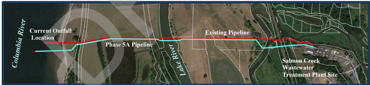
Existing (red) and Future (blue) Salmon Creek Treatment Plant Effluent Pipeline/ Outfall in Columbia River
