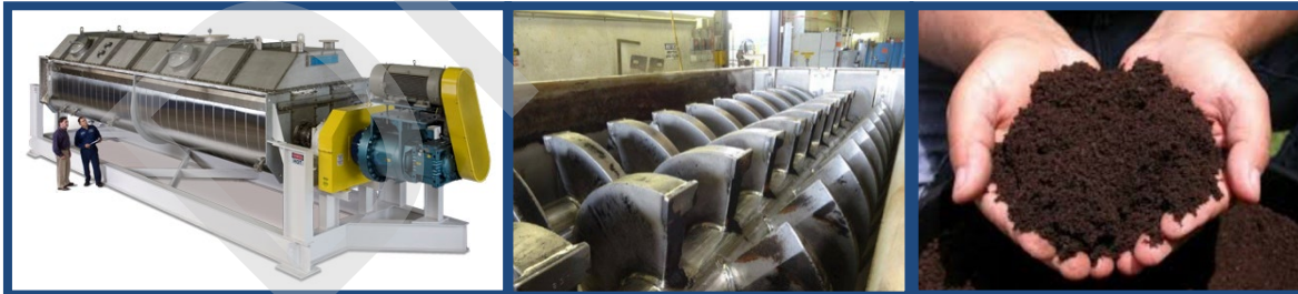
Paddle Dryer - Exterior View
