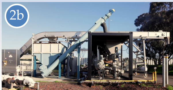
Pyrolysis Oxygen deficient, high-heat treatment
