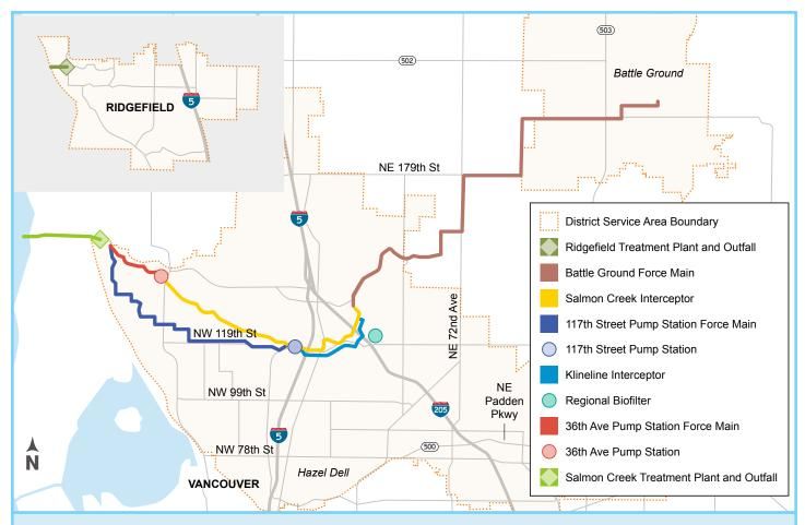
The GSP will evaluate and plan upgrades for wastewater system infrastructure such as gravity interceptors, pump stations, force mains and the Salmon Creek Treatment Plant and Ridgefield Treatment Plant.
