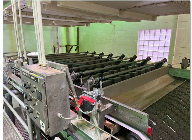
Dewatering of digested sludge occurring on the belt filter press.
