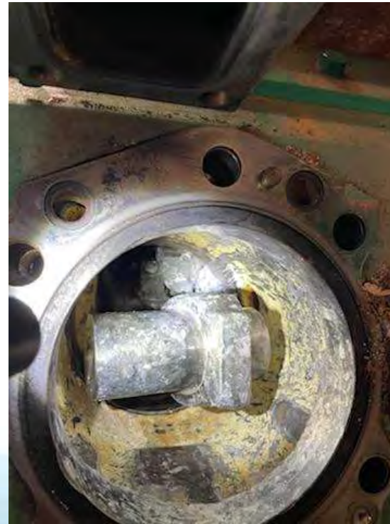
Engine Piston Failure
