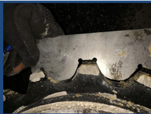
Tooth Wear on Existing NCS-720S Idler Sprockets
